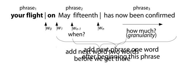
both lower lookahead and finer granularity help to reduce processing delays
