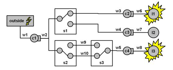
The figure above shows the electrical wiring of a fictional building, the following abbreviations are used: l = lamp, w = wire, c = circuit breaker (Sicherung), s = switch. For the first part of this assignment, you can assume that all elements work as intended.
