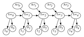
$S_t$  robot location at time t $D_t$  door sensor value at time t $L_t$  light sensor value at time t
