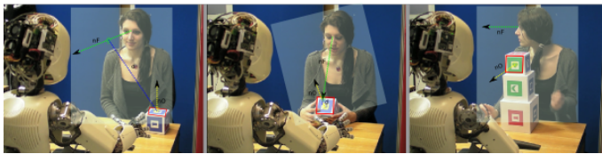
Fig. 1. Classification of the tutor’s gazing behavior: a) tutor gazing towards the robot, b) tutor gazing towards the object and c) tutor gazing elsewhere
